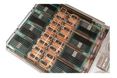
Water Cooled for energy efficiency
