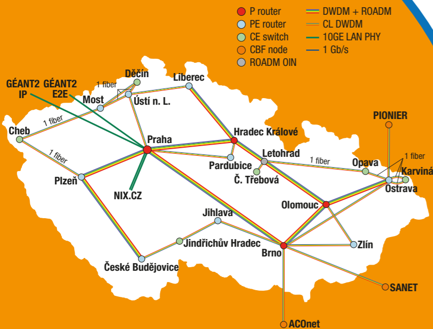
Figure 2: Basic optical topology of the CESNET2 backbone network
