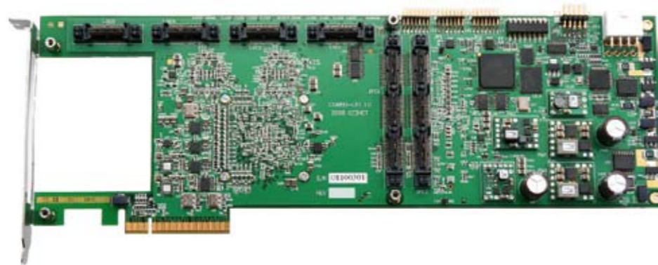
Fig. 2 – COMBO10G4TXT interface card with four 10 GE ports
