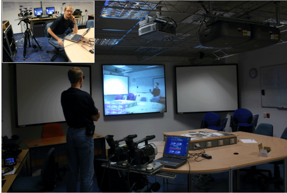
Figure 10.1: Stereoscopic video transmission using DV over IP and stereo-projection
