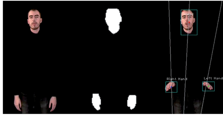
Fig. 1. a) source frame from the camera, b) segmented image c) head and hands tracking
